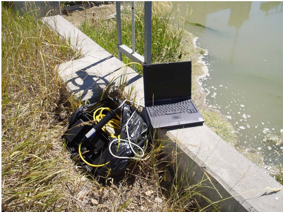
Figure 2-4. Portable Data Logger and Laptop Installed at the 12.5 Lateral Head Gate.
