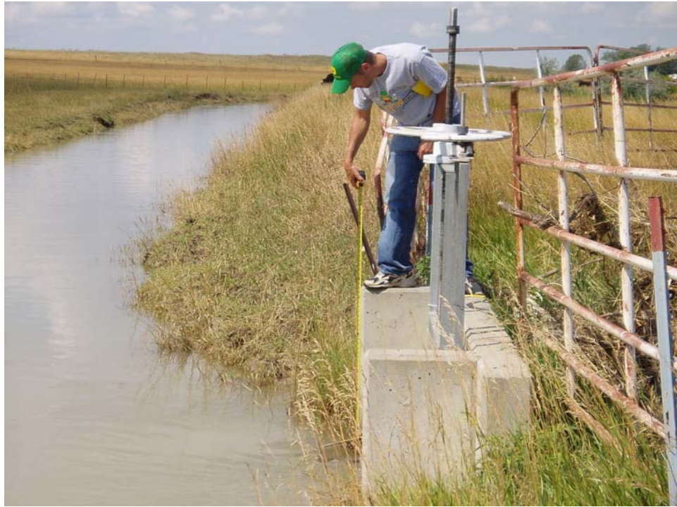
Figure 2-6. Field Monitoring Measurement at a Lateral Head Gate.
